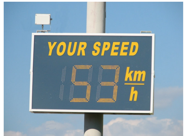
Figure 1: A speed indicator display, connected to the GSM/GPRS network. Above the upper left corner, there is a radar detector. The GSM/GPRS modem and the antenna are installed within the casing of the device.
